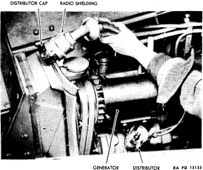
Figure 80 — Removing Distributor Cap and Radio Shielding - (Gasoline Engine)
