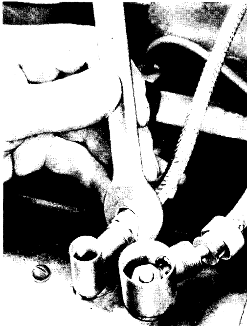
Figure 107 — Removing Coupling Nut on Field Terminal
