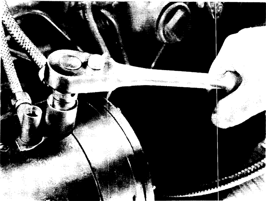
Figure 104 — Removing Armature Terminal
