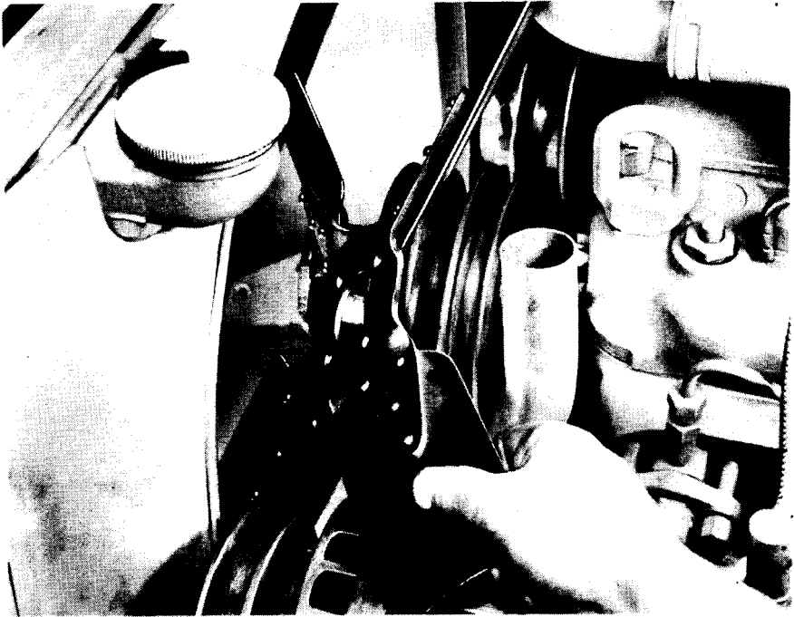
Figure 57 — Removing Fan Blade from Engine Compartment - (Hercules Diesel)
